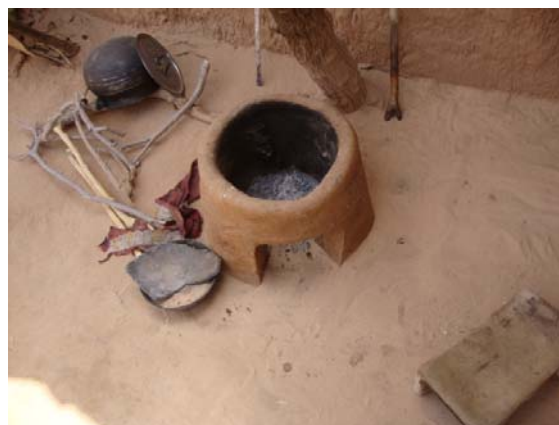
The use of the 'Albarka,' a fuel efficient cook stove, further reduces pressure on the ecosystem that is weakened by the effects of climate change. It also protects community members against fires, especially given the high winds blowing in Tamalolo.
